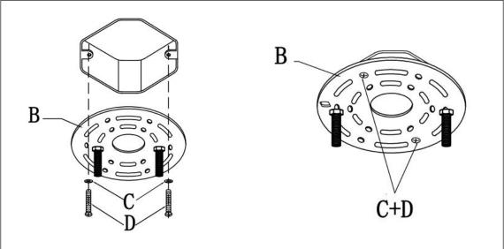
3. Turn **off** the **Power** first, Attach Mounting Plate **(B)** base to electrical junction box using Head Screws**(D)** and Washers **(C)** provided in hardware package.
