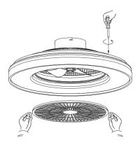
Note: Do not flush the lamp body with water directly. After the fan lamp is cleaned, please dry it first. To avoid the risk of falling, please confirm the parts are installed correctly.
