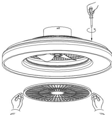
Note: Do not flush the lamp body with water directly. After the fan lamp is cleaned, please dry it first. To avoid the risk of falling, please confirm the parts are installed correctly.
